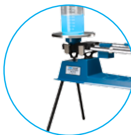
Tripod legs and integral weigh-below hook make density experiments convenient and easy.
